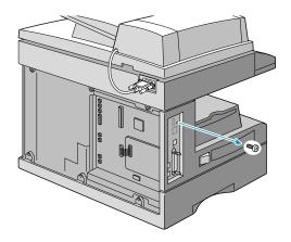
6 Remove the port cover by using your finger or a screw driver from the machine.
